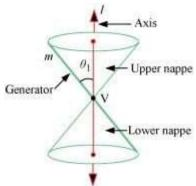
Here, the fixed line l is called the axis of the cone and m is called the generator of the cone. The intersection (V) of l and m is called the vertex of the cone.
